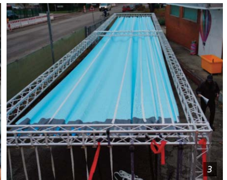
Figure 1. The Arc de Triomphe wrapped in 25.000m 2 of recyclable polypropylene silvery blue fabric with 3.000m of red ropes. Figure 2a/b. First large scale mock-up. Figure 3. Vault tensioning test for 23m free span at geo die Luftwerker. Figure 4a. Patterning the fabric. 1:20 corner mock-up built at bfl office. Figure 4b. 1:3 mock-up at Gerüstbau Tisch GmbH. Figure 5a/b. Installation test with the unrolling of the fabric.
